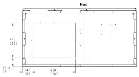
Figure 3-6. ISBM Section Dimensions (Bottom View)
